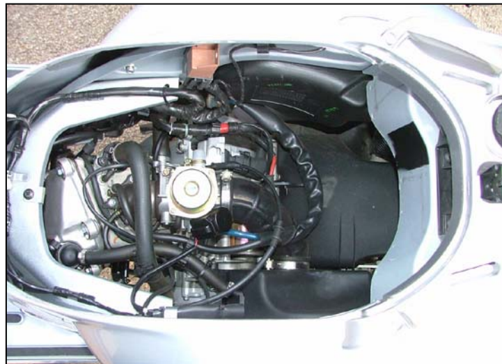
Fig. 1.3: GT200 internal combustion engine (ICE), shown with the seat and helmet storage removed
