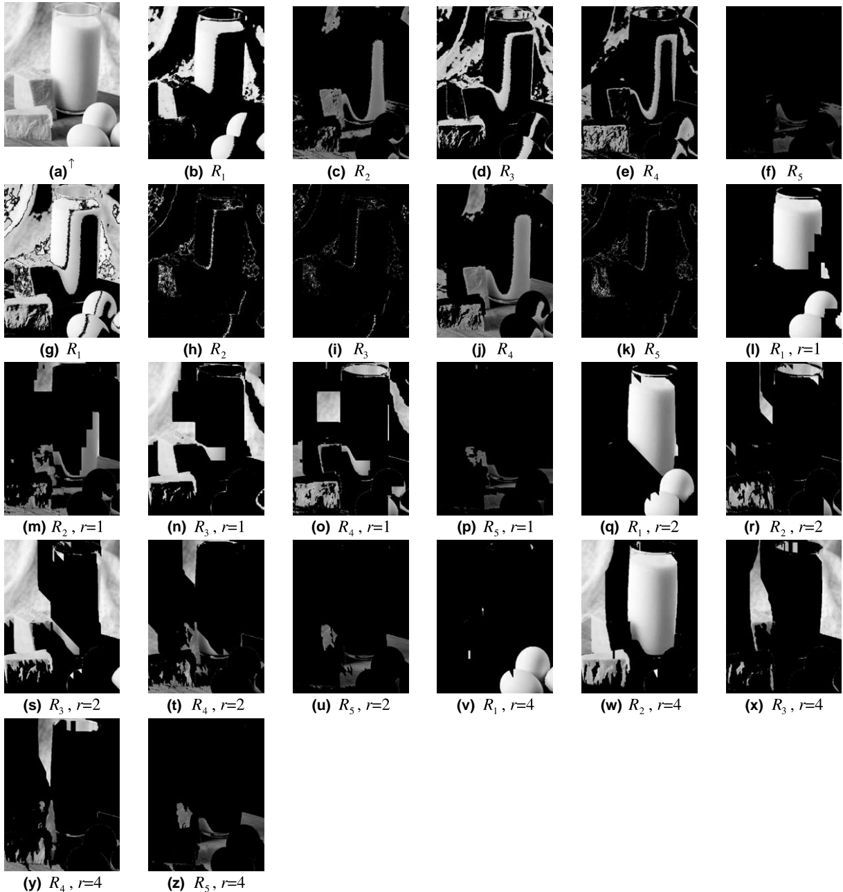
Fig. 6. Original food image (a), and its segmented results for five regions produced by FCM (b)–(f), PCM (g)–(k), and GFRIS (l)–(z).
