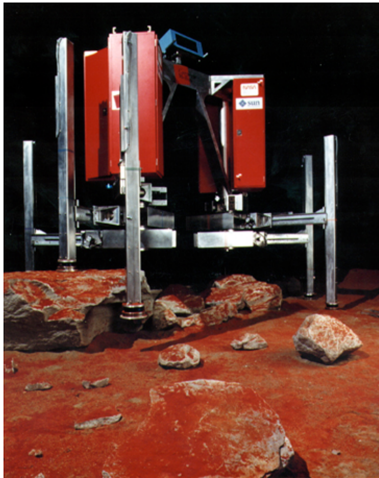
Fig. 11: The Ambler robotic walker.
