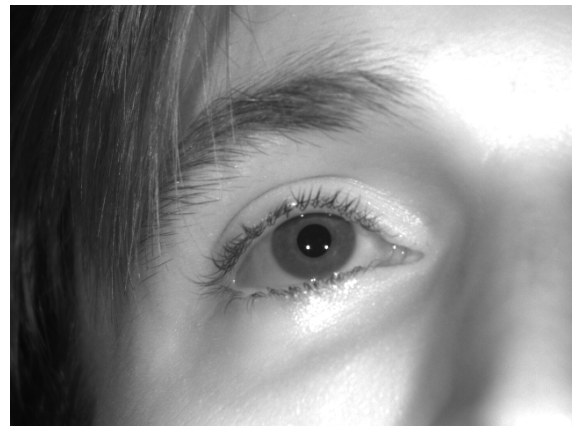
(b) Sample eye image showing the pupil and the two corneal reflections (glints)
