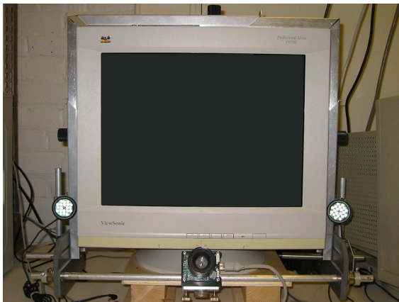
(a) System setup showing the video camera and the IR light sources
