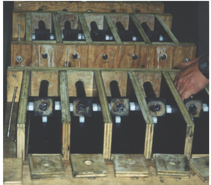
Figure 5. Moulds for the prisms
