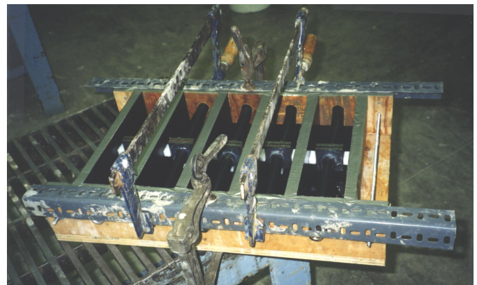
Figure 7. Moulds ready for casting
