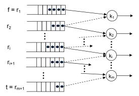
Figure 2: A sequence of m server interchanges (reallocations) results in a feasible packet interchange I(f,t). The dotted line denotes original server allocation. The solid line denotes server reallocation that implements I(f,t).
