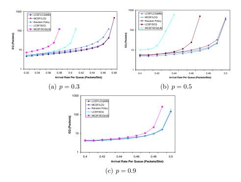
Figure 6: Average total queue occupancy, EQ, versus load under different policies, L=8 and K=4.
