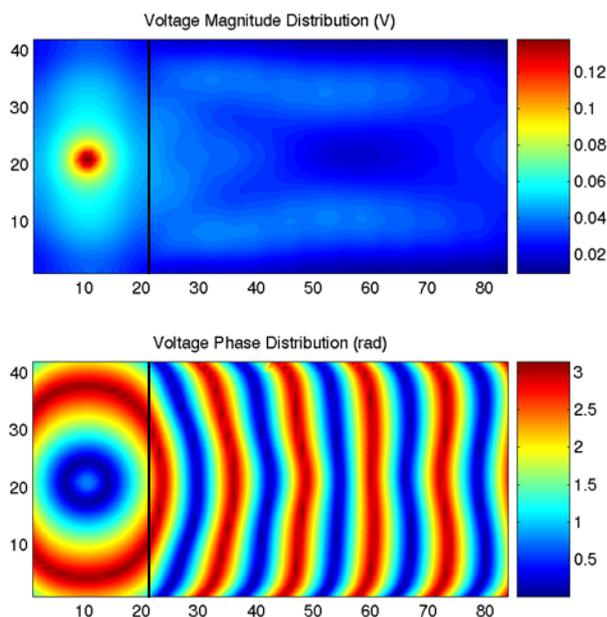
Fig. 5: Point source illuminating a RHM1/RHM2 interface at 2 GHz (relative refractive index +2, finite air-filled transmission lines with  $\Delta d=5\text{mm}$  included in each unit cell), no focusing observed in either phase or magnitude; the axes are labeled according to cell number.
