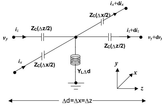
Fig. 2: 2-D Loaded High-Pass Transmission Line Unit Cell
