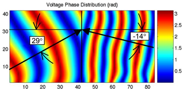
Fig. 3: Plane wave illuminating a RHM/LHM interface at 2 GHz (relative refractive index  $-2$ , homogeneous limit with  $\Delta d \ll \lambda$ ), negative refraction observed; the axes are labeled according to cell number, and the right vertical scale designates radians.
