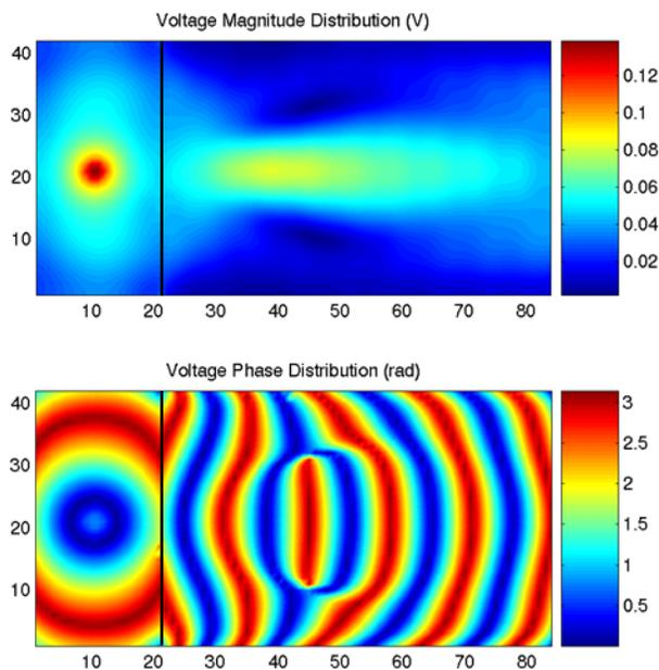
Fig. 6: Point source illuminating a RHM/LHM interface at 2 GHz (relative refractive index -2, finite air-filled transmission lines with  $\Delta d =5\text{mm}$  included in each unit cell), focusing observed in both phase and magnitude; the axes are labeled according to cell number.
