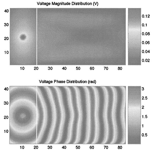
Fig. 10. Point source illuminating an RHM1/RHM2 interface at 2 GHz (relative refractive index  $+2$ , finite air-filled transmission lines with  $d = 5$  mm included in each unit cell). No focusing was observed in either phase or magnitude. The horizontal axis is labeled according to cell number.
