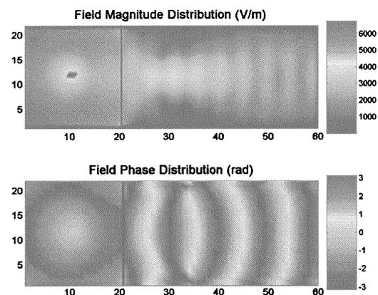
Fig. 13. Vertical electric-field distribution due to a voltage source illuminating the interface between an unloaded transmission-line grid (RHM with  $n = +2.25$ ) and a dual  $L-C$  loaded grid (LHM designed for  $n = -5.5$ ) with periodicity  $d = 5$  mm and relative permittivity of space  $\epsilon_r = 2.53$ ; The horizontal axis is labeled according to cell number.
