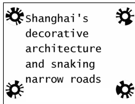
Figure 2.6: Sample reading card with circular coded targets placed at the corners.
