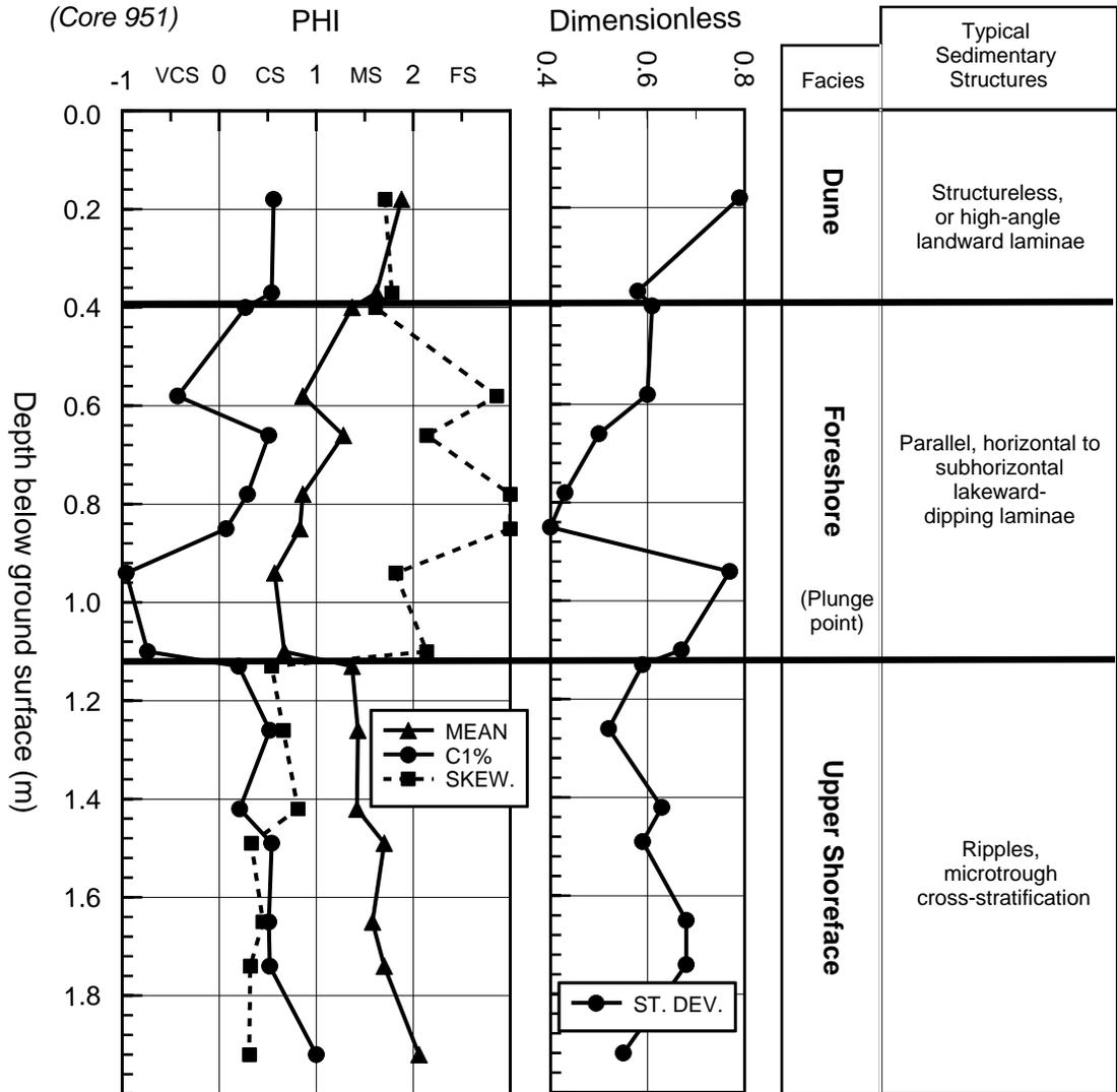
Fig. 1.3 Schematic diagram illustrating facies grain-size characteristics in core 951 with respect to depth and typical sedimentary structures in all cores. See Fig. 2 for grain-size abbreviations.
