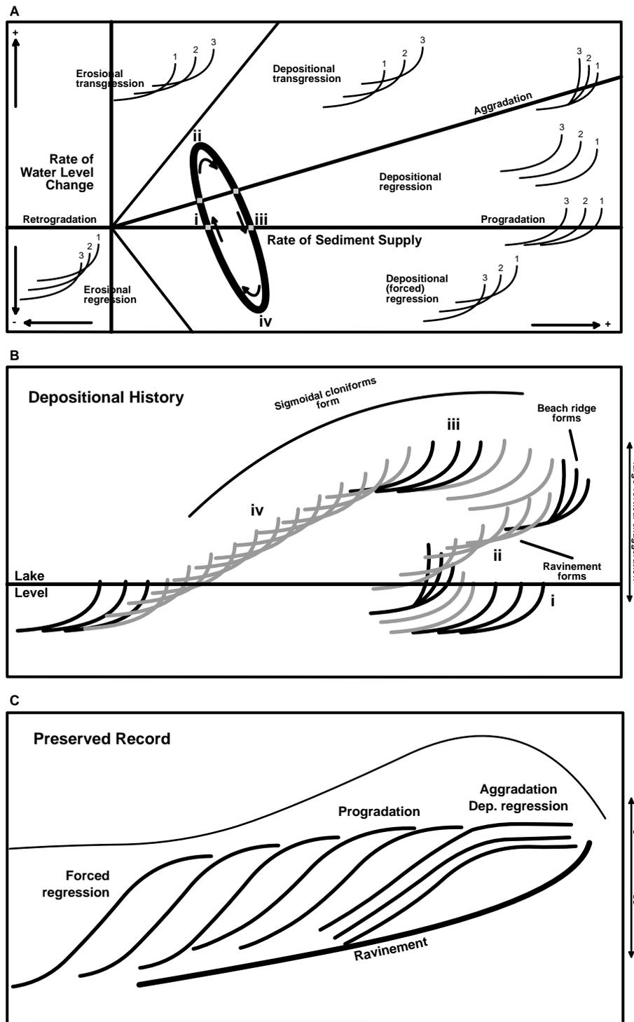
Figure 2.3 Model of (A) beach-ridge development, (B) depositional history of equilibrium profiles during a rise and fall in water level, and (C) potential sequence developed during the creation of a single beach ridge.
