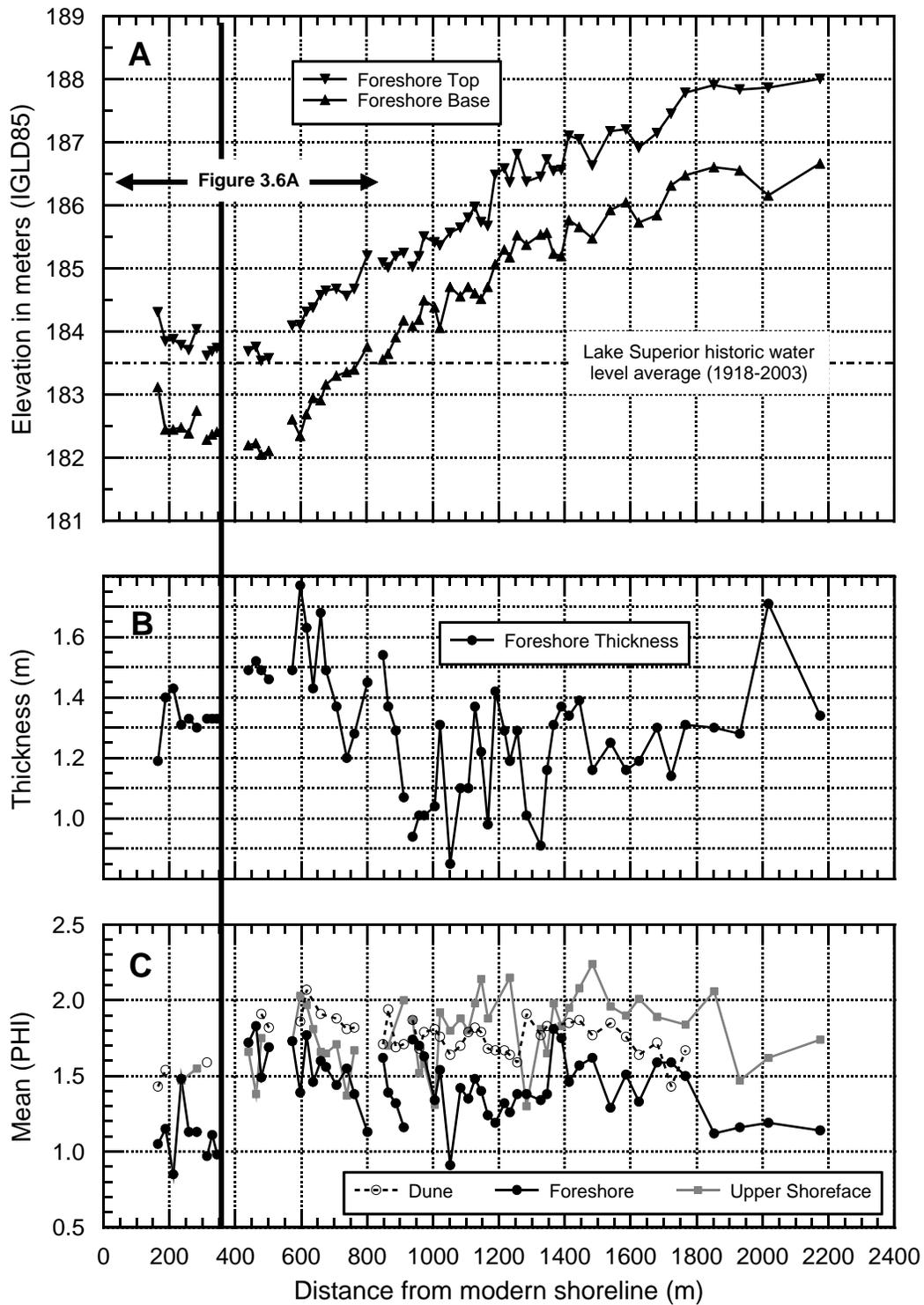
Figure 3.2 Graphs of A) facies contact elevations, B) foreshore thickness, and C) mean grain size per facies from the Grand Traverse Bay strandplain in Michigan. Gaps in data sets are locations where beach ridges were not cored.
