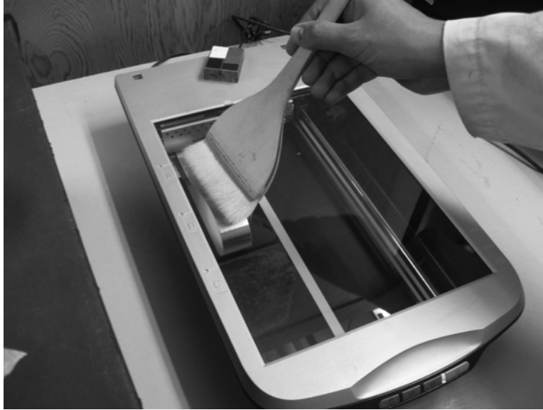
Figure 17: Removing dust from scanner plate glass using soft brush.
