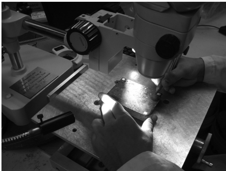
Figure 16: Darkening of micro-sized voids in aggregate using marker.
