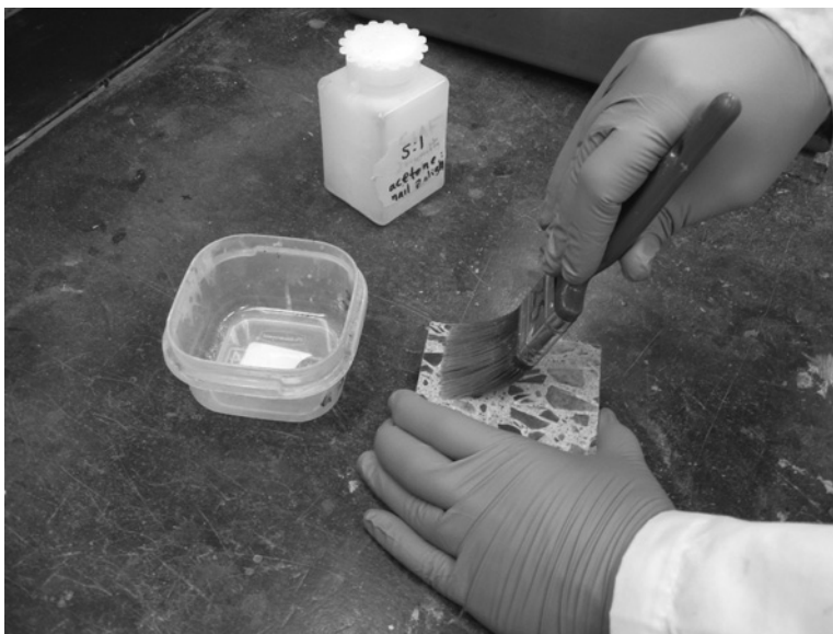
Figure 8: Application of nitrocellulose solution to strengthen paste matrix.
