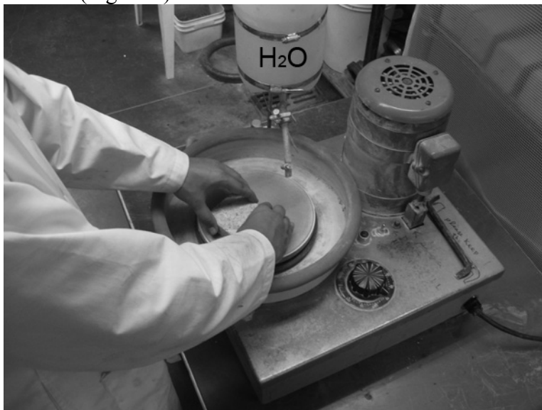
Figure 2: Surface grinding with water and diamond embedded platen.
