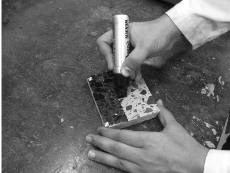
Figure 12: Darkening the surface with marker.
