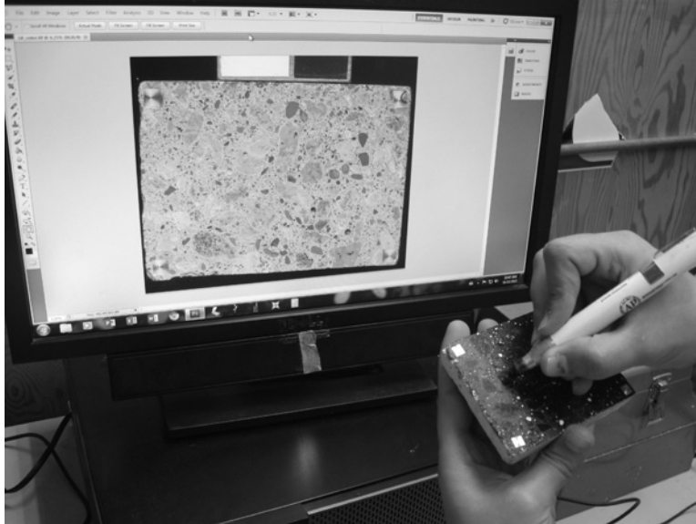
Figure 15: Darkening of macro-sized voids in aggregate using marker.
