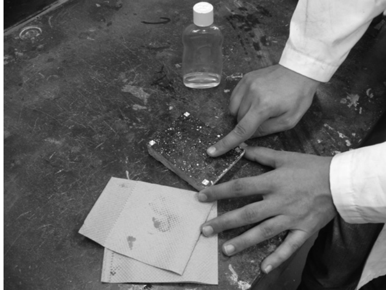
Figure 14: Wiping of excess powder with lightly-oiled fingertip.
