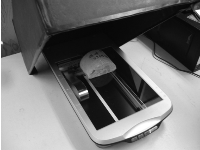
Figure 19: Covering scanner with light-proof non-reflective black-interior box prior to image collection.
