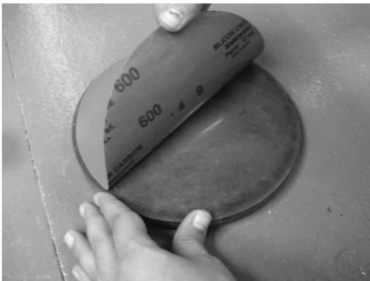
Figure 9: Mounting PSA SiC paper to grinding wheel platen.
