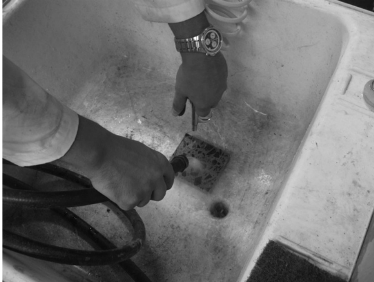
Figure 3: Cleaning the surface with combined water and compressed air.
