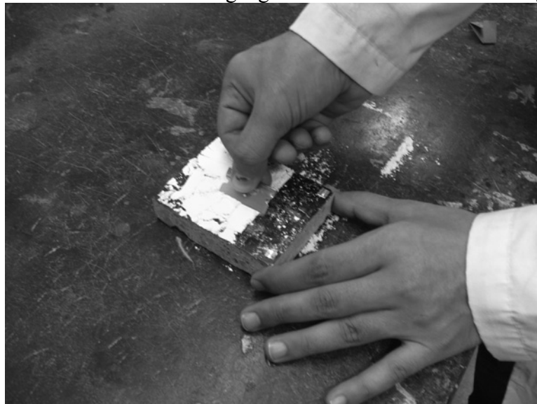
Figure 13: Removal of excess powder with razor blade.
