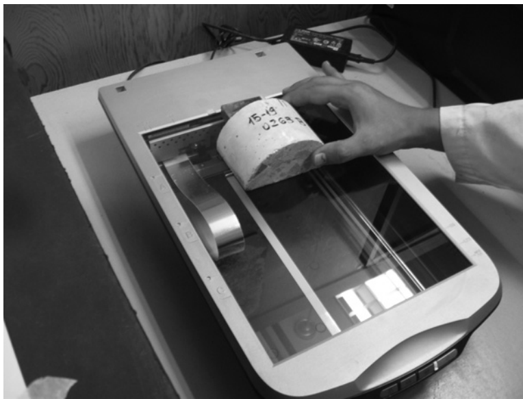
Figure 18: Gently placing sample face down on scanner plate glass.
