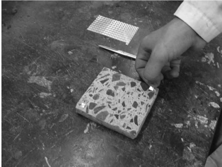
Figure 11: Application of stickers (cut from sheet) to four corners.
