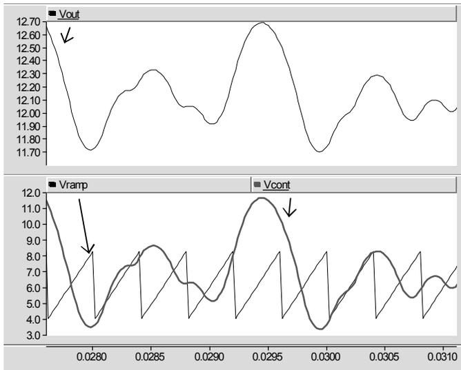
Fig. 8. Plot of output voltage, ramp generator output, and the control voltage vs. time for the chaotic operation with  $E = 33$  V.
