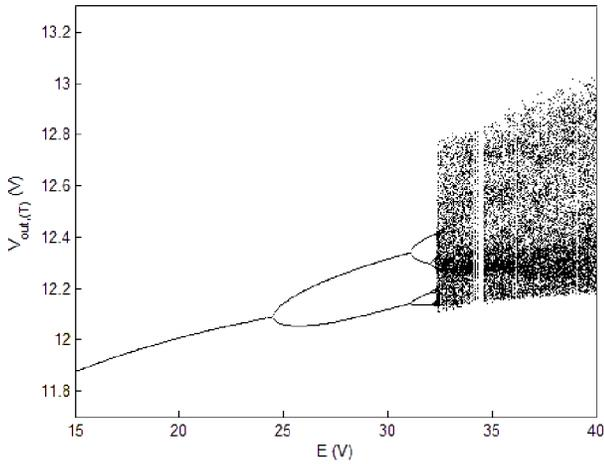
Fig. 4. Bifurcation diagram obtained by sampling the output voltage at the end of each cycle.
