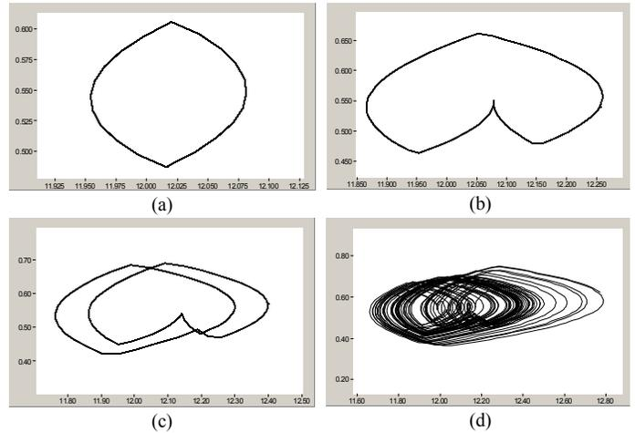
Fig. 7. Phase-space diagrams (output voltage on  $x$ -axis, inductor current on  $y$ -axis) of the PSCAD run for (a)  $E = 24$  V showing periodic operation, (b)  $E = 28$  V showing period-2, (c)  $E = 32$  V showing period-4, and (d)  $E = 33$  V showing chaotic operation.
