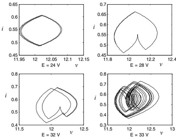
Fig. 5. Phase-space diagram of buck converter showing period-1 ( $E = 24$  V), period-2 ( $E = 28$  V), period-4 ( $E = 32$  V), and chaotic ( $E = 33$  V) waveforms obtained from numerical integration. Note jitters for  $E = 24$  and  $32$  V.
