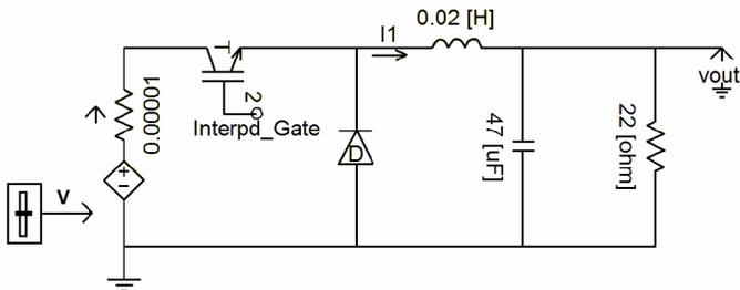
Fig. 6. PSCAD model of the buck converter.
