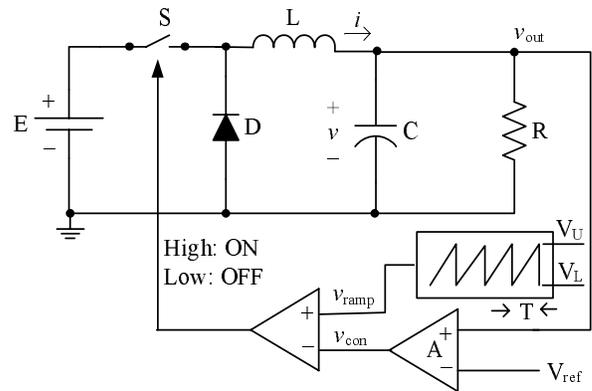
Fig. 1. Schematic of the second-order buck converter with simplified control circuitry.
