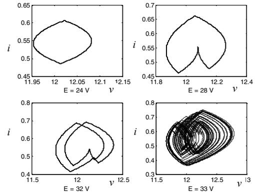
Fig. 2. Phase-space diagram of the buck converter showing period-1 ( $E = 24$  V), period-2 ( $E = 28$  V), period-4 ( $E = 32$  V), and chaotic ( $E = 33$  V) waveforms obtained from the exact solution.
