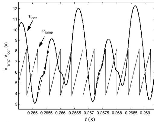
Fig. 3. Chaotic operation of the buck converter obtained by exact solution with  $E = 33$  V (shown are  $v_{con}$  and  $v_{ramp}$ ).
