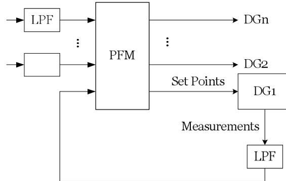
Figure 3. Potential function minimizer
