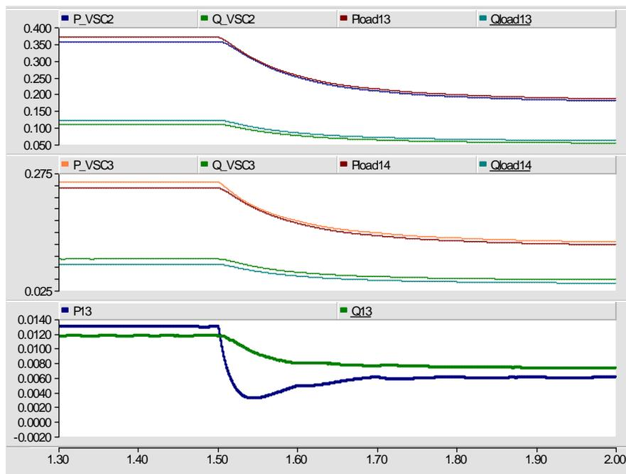
Figure 6. Case study 1: The microgrid response (power flows) to a step change in voltage
