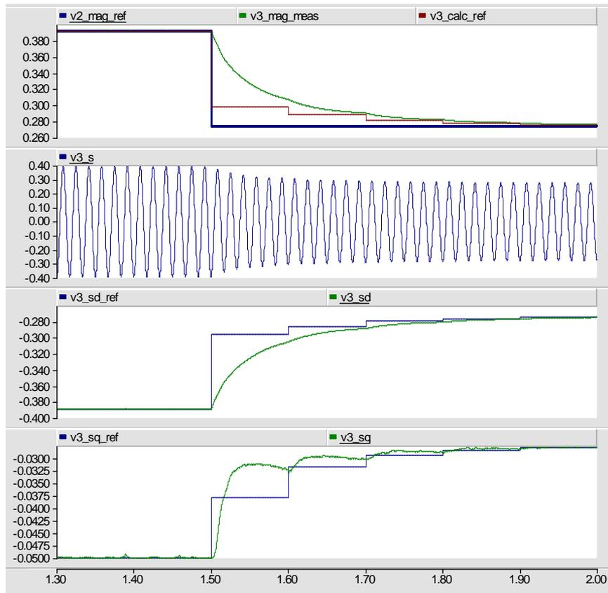
Figure 5. Case study 1: The microgrid response (voltages) to a step change in voltage
