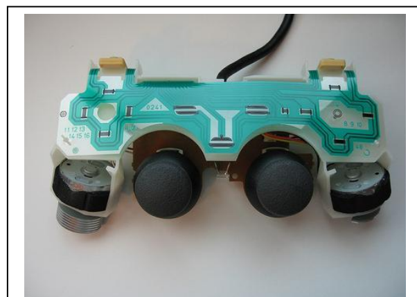
The Printed Circuit Foil, Joysticks and motors
