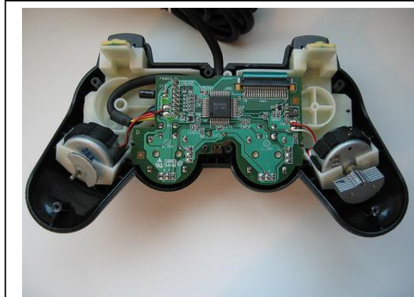
The Printed Circuit Board with an Integrated Circuit 16-pin ribbon connection and motors
