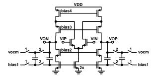
Folded-cascode op-amp with switched-capacitor common-mode feedback
