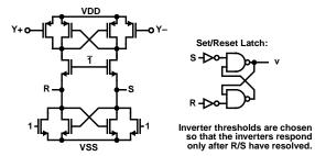
S and R connected to a Set/Reset latch.
