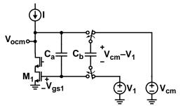
$\begin{array}{cc} \bullet & V_{ocm} = V_{cm} + V_{gs1} - V_1 \\ & \text{If } V_1 = V_{gs1}, \text{ then } V_{ocm} = V_{cm}. \end{array}$
