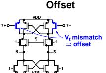
Obvious sources of offset include mismatch in the input differential pair as well as mismatch in the regenerating devices
