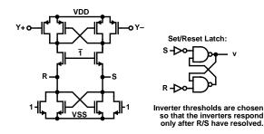
• Falling phase 1 initiates regenerative action S and R connected to a Set/Reset latch.
