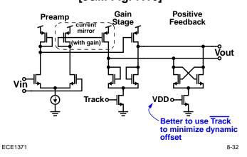
**Two-Stage Comparator** [J&M Fig 7.17] current Reset Ц Vout Vin Ŧ Reset C Positive Logic-level Preamp Feedback Restoration
