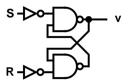
Inverter thresholds are chosen so that the inverters respond only after R/S have resolved.
