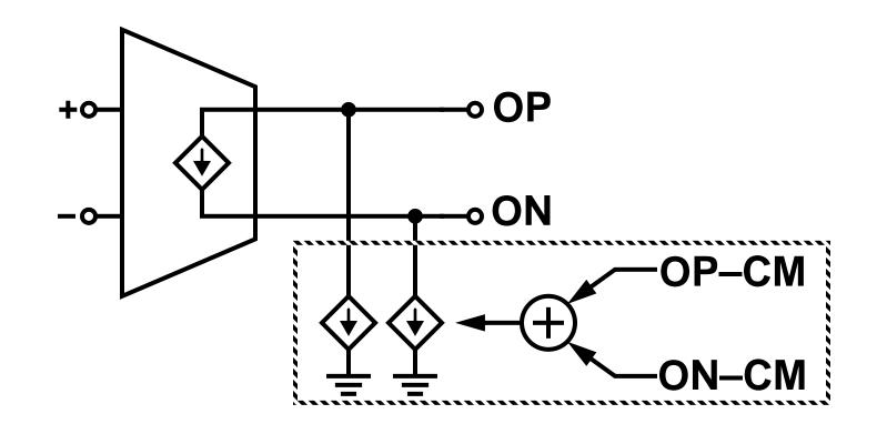
• Can use this circuit to speed up the simulation
