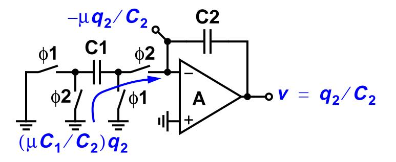
• A fraction of  $q_2$  leaks away each clock cycle:
