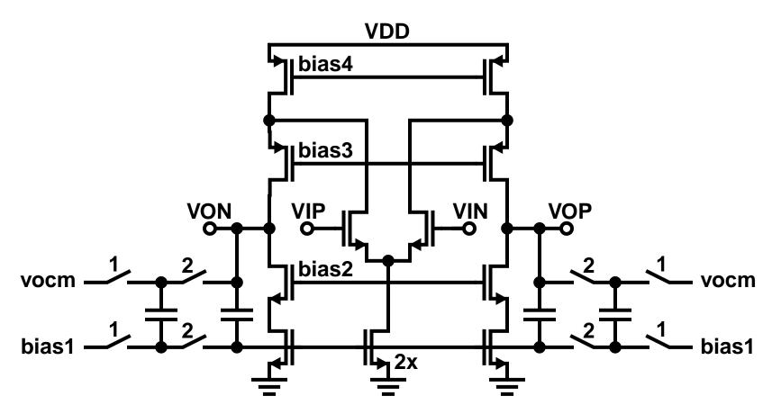
Folded-cascode op-amp with switched-capacitor common-mode feedback
