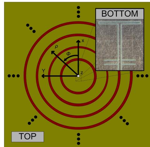
Fig. 1. The planar ‘bull-eye’ LWA considered in this work defined by annular periodic metallic strip gratings on a GDS. A slotted magnetic dipole source, realized by a non-directive SWL [6], acts as the practical antenna feed.
