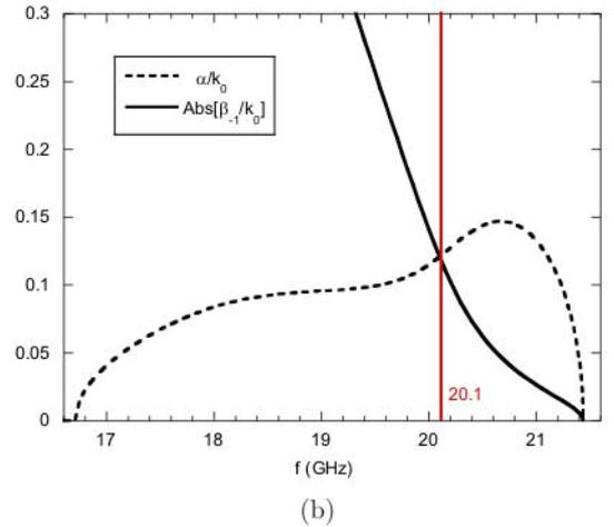
Fig. 3. (a) Brillouin diagram for the MSG printed on a GDS ( $\epsilon_r = 10.2$ ) with thickness  $h = 1.27$  mm, and period  $d = 7$  mm. The strip width is  $w = 1.25$  mm. (b) Phase (solid line) and attenuation (dashed line) constants normalized to the free-space wavenumber as a function of frequency for the same structure as in (a).
