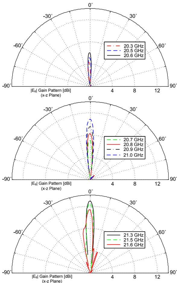
Fig. 4.  $E_{\theta}(\phi = 0^{\circ})$  gain patterns (in the  $x-z$  plane) for the LWA structure. A broadside beam is first observed at 20.5 GHz and a maximum is achieved at  $f_{b,max} = 21.3$  GHz. Gain reduces with an increase in frequency.
