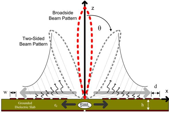
Fig. 2. By the addition of concentric metallic strips grating (width,  $w$  and pitch,  $d$ ) LWs can be excited on the planar guiding surface generating broadside ( $f = f_b$ ) or two-sided beam patterns ( $f \gg f_b$ ) in the far field.
