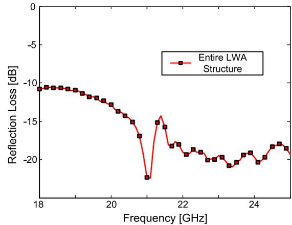
Fig. 5. Simulated reflection loss values for the investigated LWA design.
