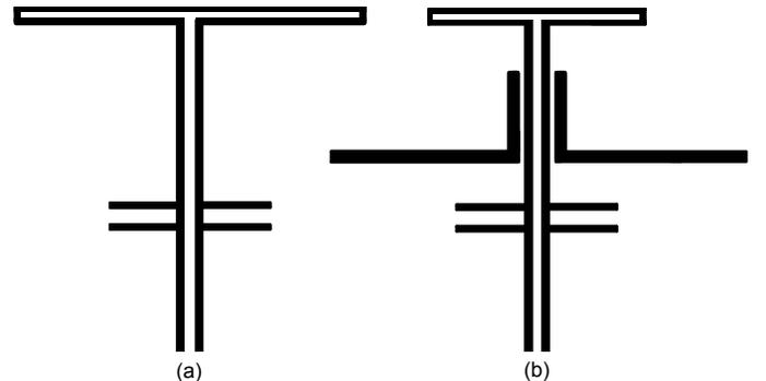
Fig. 4. Ground plane trace of the utilized (a): non-directive [8] and (b): directive [10] SWL sources; realized by ground plane slots in the base slab ( $\epsilon_{r_1}, h_1$ ). Main top ‘T’ slot lengths are 2.5 mm and 2.0 mm, respectively.
