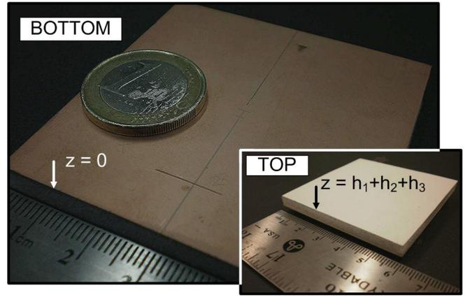
Fig. 3. Measured 6 cm by 6 cm multilayer LWA ( $\epsilon_{r_i}=[10.2, 1, 30]$  and  $h_i=[1.27, 3, 0.7874]$  mm) with a non-directive SWL in the ground plane.
