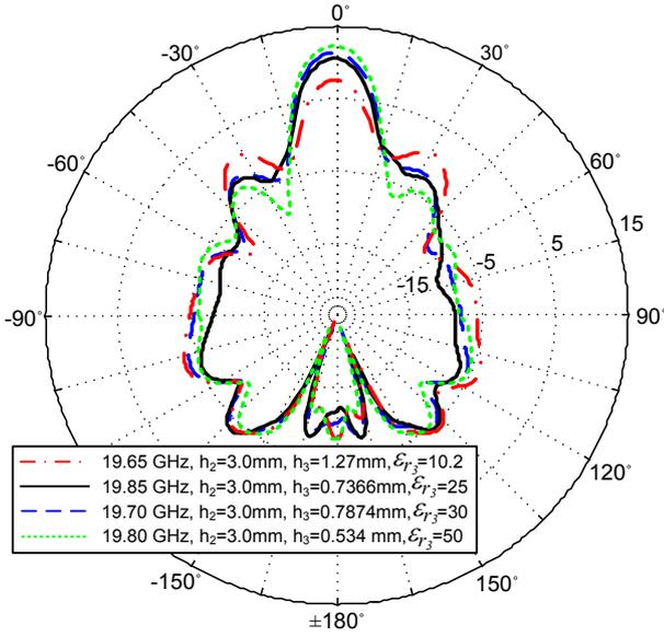
Fig. 5. Simulated  $E_\theta(\phi = 0^\circ)$  gain patterns in the  $E(x-z)$  plane (in dBi) using a single non-directive SWL. Observed maximum gain values are shown. Improved gain is possible by increasing  $\epsilon_r$  of the top dielectric layer.
