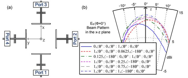
Fig. 10. (a): Investigated SWL array for broadside beam steering and CP. (b): By the appropriate feeding the main far field beam can be steered  $\pm 4.5^\circ$ . Substrate parameters  $\epsilon_{r_i}=[10.2, 1, 25]$  and  $h_i=[1.27, 3.0, 0.7366]$  mm.
