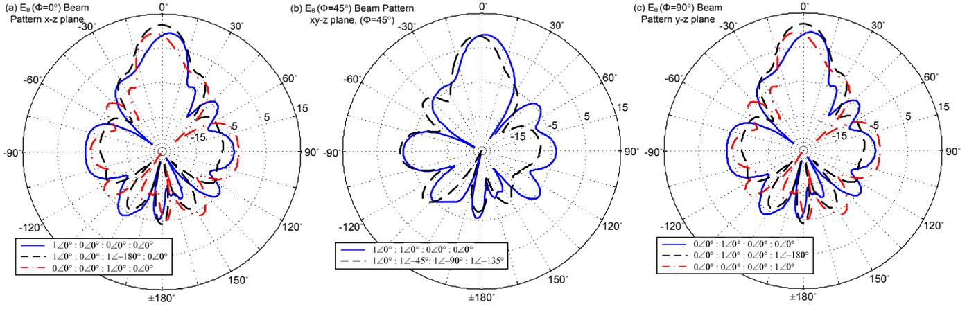
Fig. 11. Broadside beam steering at 19.85 GHz by tuning the feeding array distribution. The main pencil beam can be contained and controlled within a small cone defined by  $\theta \in \pm 4.5^\circ$  and  $\phi \in \pm 180^\circ$ . Simulated results are shown in dBi in the  $x-z$  ( $\phi = 0^\circ$ ),  $xy-z$  ( $\phi = 45^\circ$ ), and  $y-z$  ( $\phi = 90^\circ$ ) planes.
