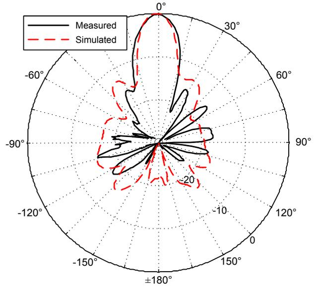
Fig. 7. Measured beam patterns in the  $E(x-z)$  at 17.4 GHz and normalized to observed maximum gain. Values shown in dB. Agreement can be observed with the simulated beam pattern;  $\epsilon_{r_3}=30$  and  $h_3=0.7874$  mm, as in Fig. 5.
