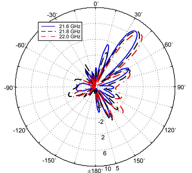
Fig. 8.  $E_\theta(\phi = 0^\circ)$  gain patterns (in the  $x-z$  plane) in dBi for the investigated LWA using a directive SWL source. A maximum of 7.15 dBi is observed at  $\theta = 40^\circ$  for  $\epsilon_{r_i}=[10.2, 1, 25]$ ,  $h_i=[1.27, 2.786, 1.27]$  mm.
