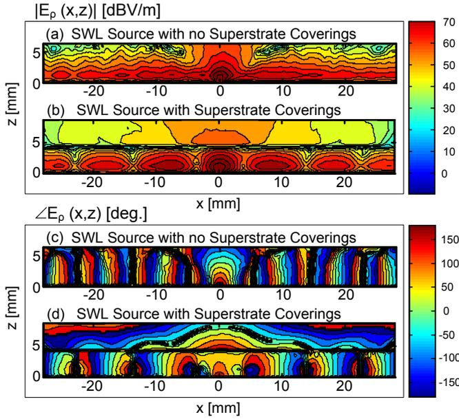
Fig. 9. Field distribution generated by the non-directive SWL source at 19.85 GHz. A comparison is made with and without the superstrate coverings. Substrate parameters  $\epsilon_{r_i}=[10.2, 1, 25]$  and  $h_i=[1.27, 3.0, 0.7366]$  mm.
