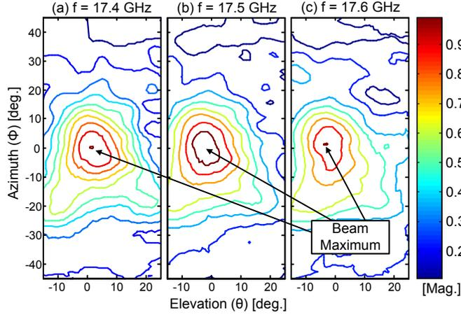
Fig. 6. Measured 2D gain patterns in the azimuth and elevation. Values have been normalized to observed maximum and results are shown in linear units.
