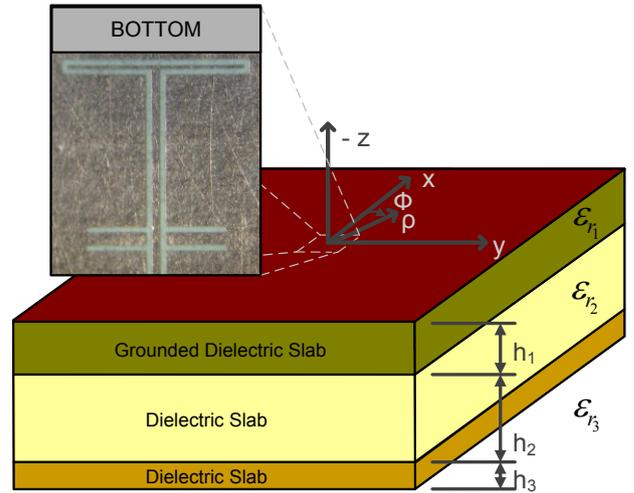
Fig. 1. Illustration of the compact LWA considered in this work defined by a base GDS ( $\epsilon_{r1}$  and  $h_1$ ) covered by two superstrate dielectrics. A single SWL or an array of sources can be utilized as the printed antenna feed.
