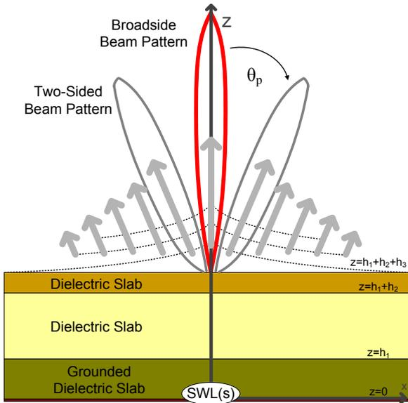
Fig. 2. Stackup configuration of the proposed multilayer LWA fed by SWL(s). By the appropriate source configuration and dielectric layers, one-sided or two-sided beam patterns are possible along with CP and beam steering. In this work all substrate dimensions were held constant to 6 cm by 6 cm.
