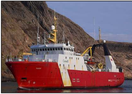
Fig. 3. Photograph of a Teleost vessel used in the Canadian Coast Guard. The length and breadth of the ship was 63 m and 14.2 m, respectively.
