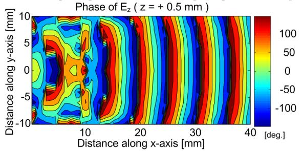
Figure 7: Simulated  $TM$  phase distribution generated on the guiding surface by a SWL source placed at the origin with the plane-wave grating lens and no strips. A bound plane-wave distribution is generated for  $x \geq 14$  mm and  $y \leq |5|$  mm.
