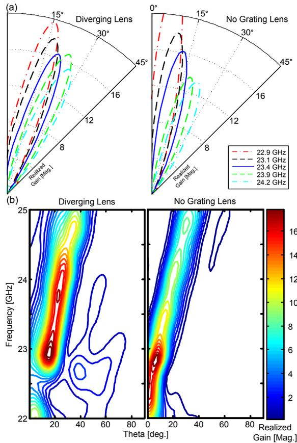
Figure 9: Beam patterns in the  $x - z$  plane for the circular strip LWAs: (a) Polar plot of the beam pattern with and without the diverging grating lens. (b) Elevation angle ( $\theta$ ) versus frequency with and without the diverging grating lens. A null is observed at broadside for both designs. Increased gain values are observed over a larger bandwidth for the lens LWA design.
