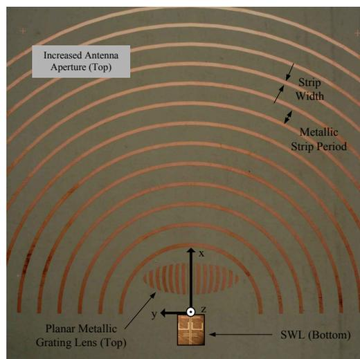
Figure 1: Realized planar LWA considered in this work. Using printed curvilinear strips on a GDS LWs can be excited (from a central SWL source) generating directive beam patterns in the far field. By the addition of a planar metallic grating lens on top of the GDS (for SW divergence) increased gain values can be observed in the far field.
