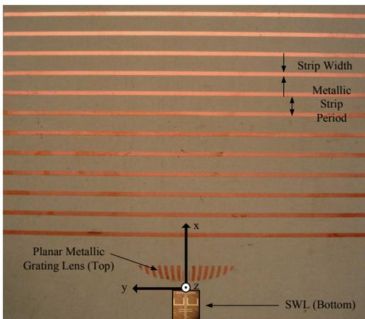
Figure 3: Planar antenna with a printed grating lens (for a linear phase front on the aperture) and straight strips.
