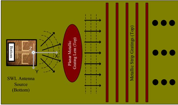
Figure 2: Illustration of the proposed LWA with printed strips. A bound plane-wave can be generated by the lens for in phase diffraction and directive beam patterns in the far field.
