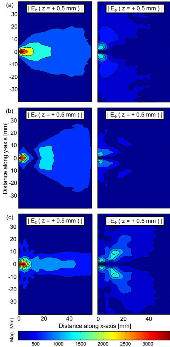
Figure 5: Simulated  $TM$  ( $E_z$ ) and  $TE$  ( $E_\phi$ ) SW field distributions generated on the guiding surface (with and without the grating lenses and no strips): (a) no lens, (b) diffracting lens and (c) plane-wave lens.
