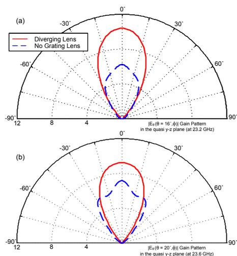
Figure 10: Beam patterns in the quasi  $y - z$  planes generated by the linear strips with and without the grating lens for bound plane-wave excitation at (a) 23.2 GHz and (b) 23.6 GHz.
