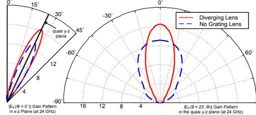
Figure 8: Comparison of far field beam patterns in the  $x-z$  and quasi  $y-z$  planes at 24 GHz for the circular strip LWAs with and without the planar metallic grating lens for SW divergence.
