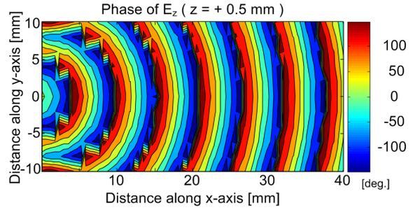
Figure 6: Simulated cylindrical  $TM$  field distribution generated on the guiding surface with no the grating lens and strips.
