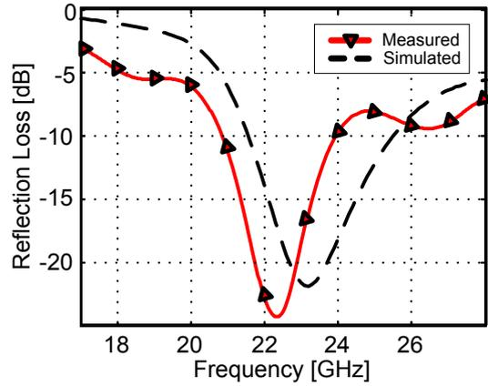
Figure 4: Reflection loss values of the directive SWL source in the antenna ground plane with no grating lenses or strips on top of the GDS.
