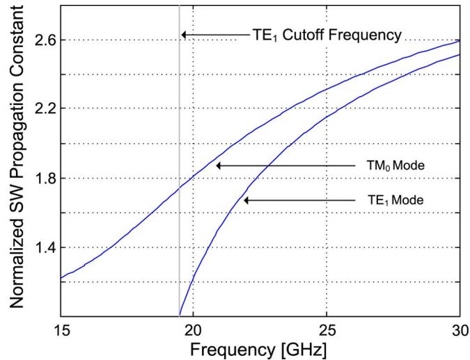
Fig. 2. SW propagation constants of the  $TM_0$  and  $TE_1$  SW modes (normalization with respect to  $k_0$ ) for the utilized GDS (with no strips). The main radiating slot [secondary reflector slots] of the SWL feed can couple power into the  $TM_0$  [ $TE_1$ ] SW mode of the slab since the  $TM_0$  SW mode has a zero cutoff frequency [ $TE_1$  SW mode can exist for  $f \geq 19.47$  GHz].
