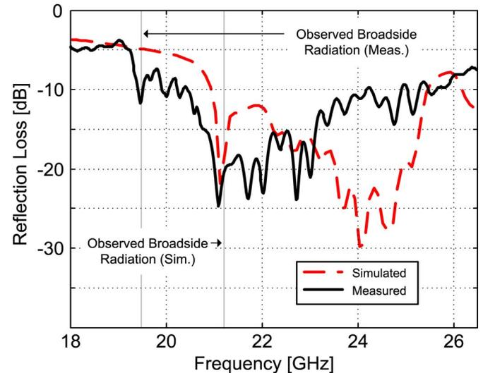
Fig. 4. Reflection loss values for the proposed LWA design with the directive SWL feed. Maximum radiation at broadside is measured [simulated] at 19.48 [21.2] GHz with loss values below 10 dB.
