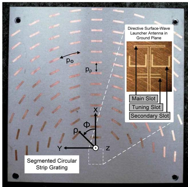
Fig. 1. Realized planar 2-D LWA. The antenna feed defined by a SWL is described by a main radiating driven slot (length of 1.92 mm) with two secondary folded reflector (individual length of 2.75 mm) and four tuning slots (individual length of 0.65 mm). A PRS is realized on top of the GDS (at  $z = 0$ ) by the addition of a segmented circular strip grating described by the periodicities,  $p_\rho$  and  $p_\phi$ , in the  $\hat{\rho}$  and  $\hat{\phi}$  directions, respectively.
