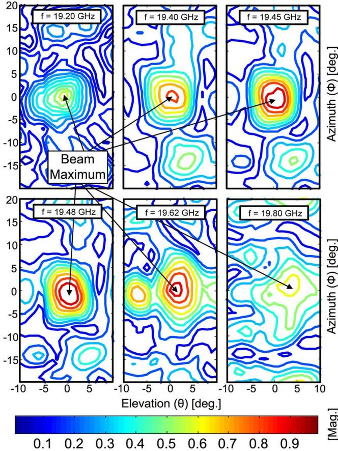
Fig. 5. Measured 2-D gain pattern in linear units and normalized to maximum gain at broadside at  $f_b = 19.48$  GHz. The pencil beam is only observed between 19.20 and 19.80 GHz and at its maximum ( $f = f_b$ ) the  $3_{dB}$  beam width is approximately  $10^\circ$  in both the azimuth and elevation.
