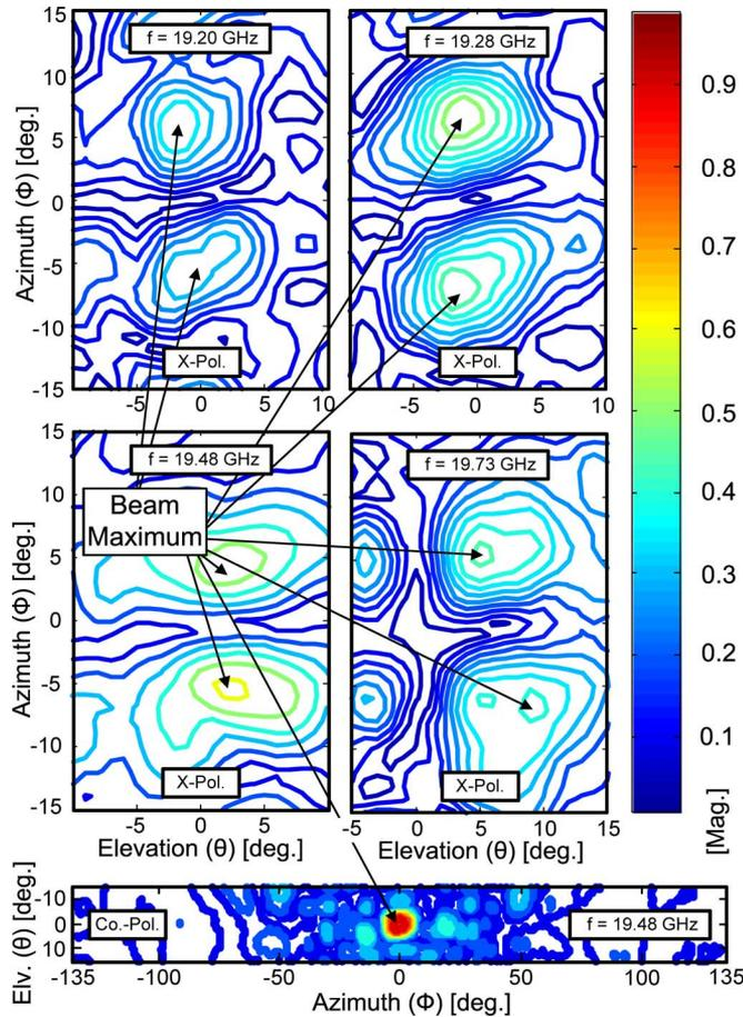
Fig. 8. Measured 2-D X-Pol gain patterns in linear units, normalized and compared to measured Co-Pol gain value ( $f_b = 19.48$  GHz at broadside).
