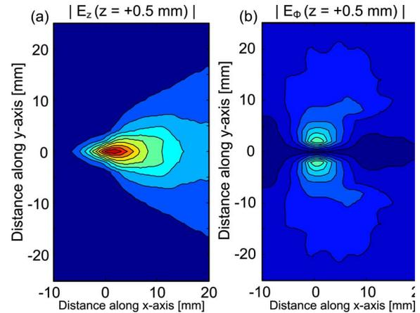
Fig. 3. Simulated TM and TE SW field distributions 0.5 mm above the guiding surface at 24 GHz: (a)  $|E_z(x, y)|$  and (b)  $|E_\phi(x, y)|$ . The majority of the TM [TE] field distribution is directed in the  $+\hat{x}$  [ $\pm\hat{y}$ ] direction[s].
