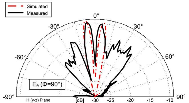
Fig. 7. Cross-polarization beam pattern at broadside:  $|E_\theta(\phi = 90^\circ)|$ . Normalized to maximum copolarization gain (Fig. 6). Values are 10 dB below the main pencil beam with a null at broadside.
