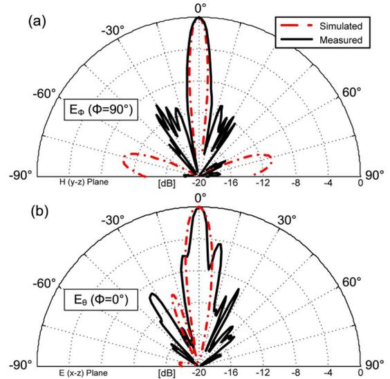
Fig. 6. Broadside beam patterns normalized and shown in dB (H/E planes referenced to main slot of SWL). (a)  $|E_\phi(\phi = 90^\circ)|$ . (b)  $|E_\theta(\phi = 0^\circ)|$ . Measured [simulated] beam patterns shown at  $f_b = 19.48$  [21.2] GHz.
