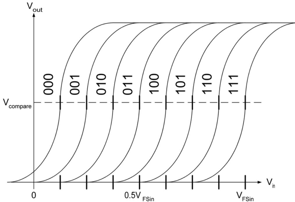
**Figure 3-1** The transfer function and output of a 3-bit interpolation ADC.
