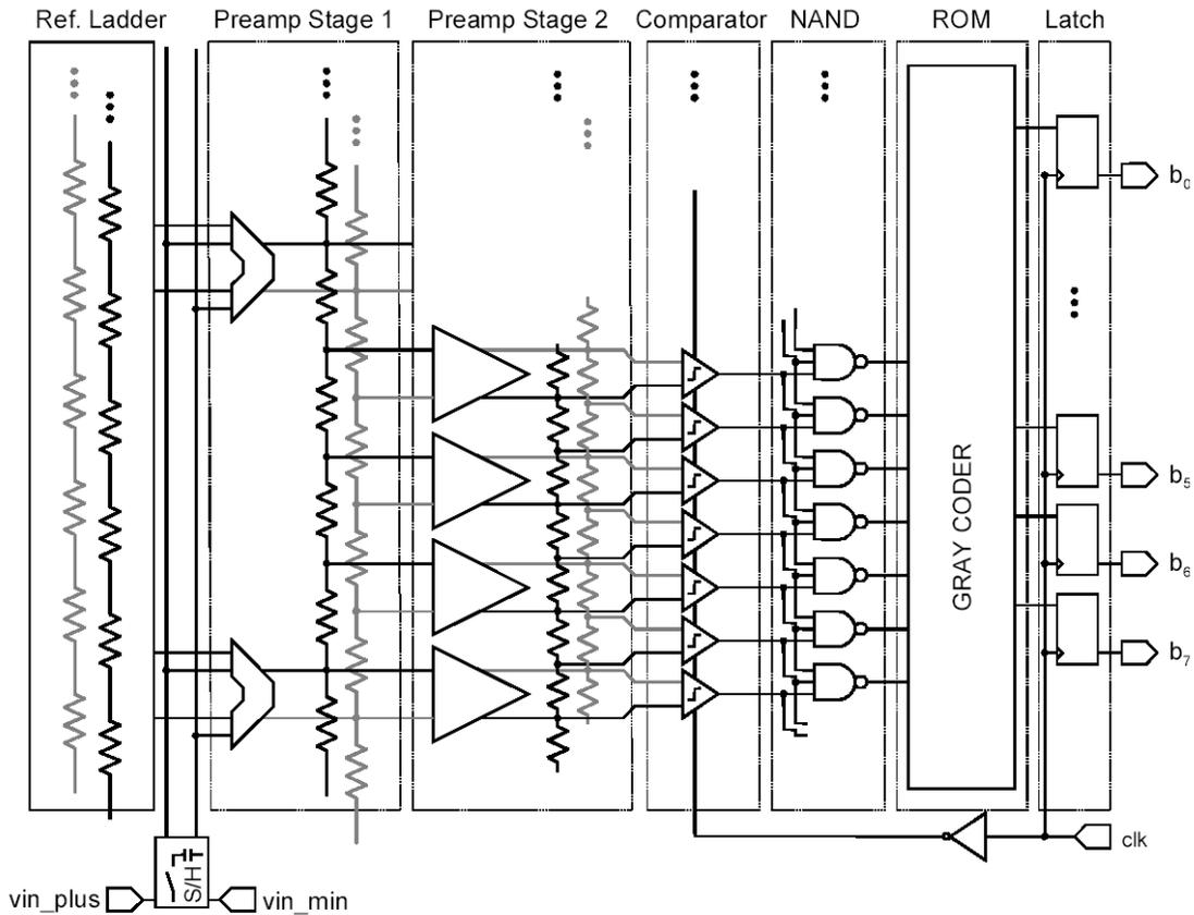
Figure 3-4 A 200 MS/s 8-bit Interpolating ADC [4].
