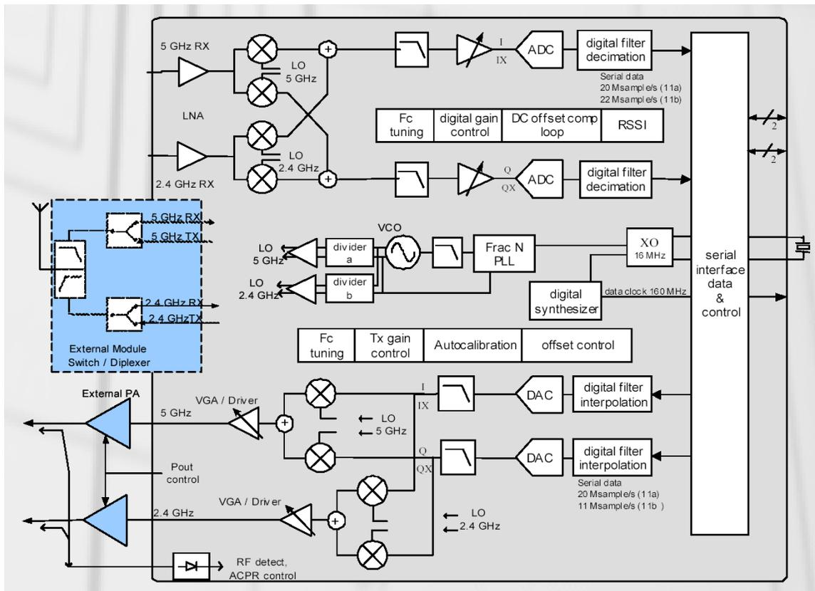
Figure 2-1 802.11a system architecture using direct conversion transceiver.
