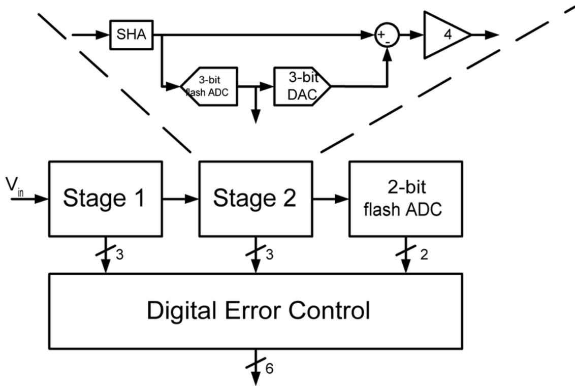
Figure 4-2 The block diagram of a 3 stage pipelined ADC with digital error control.
