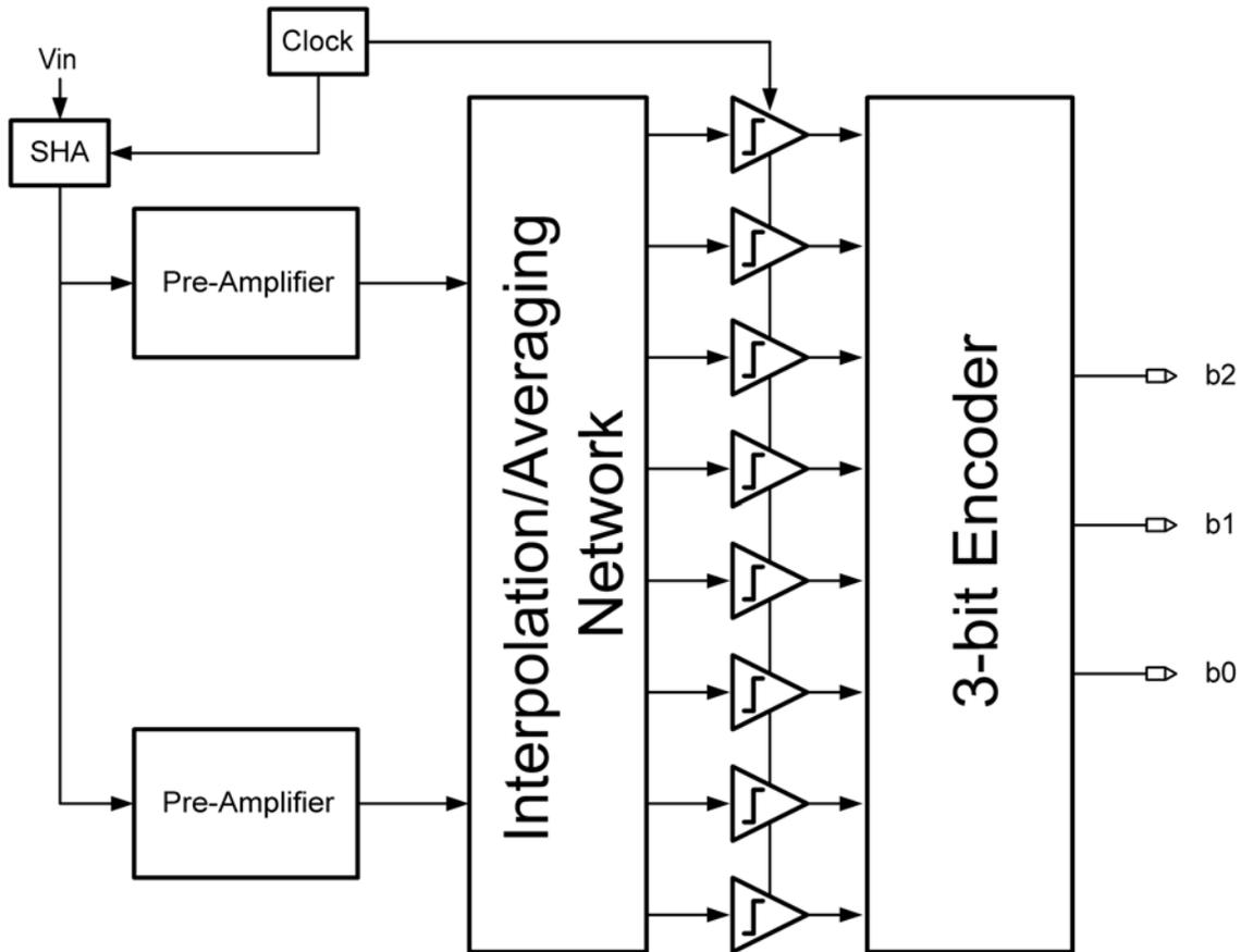
**Figure 3-2** Block diagram of a 3-bit interpolating ADC.
