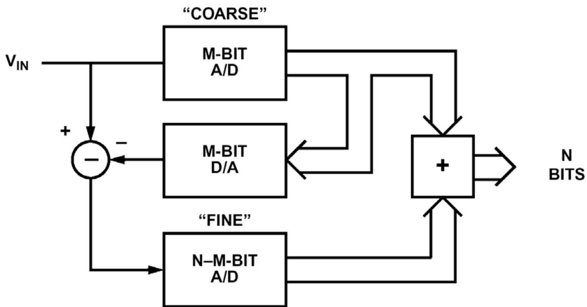
Figure 4-1 Block diagram of a 2 stages pipelined ADC.
