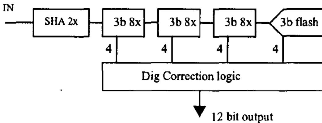
Figure 4-3 A  $115\text{mW}$  12-bit  $50\text{MS/s}$  pipelined ADC [5].
