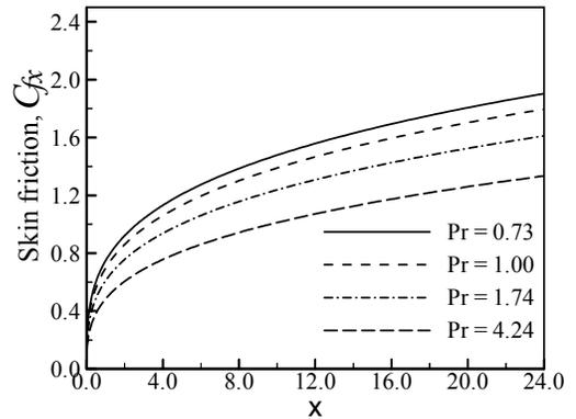
Fig 8: Variation of skin friction coefficients for different values of  $Pr$  with  $Q = 0.01$
