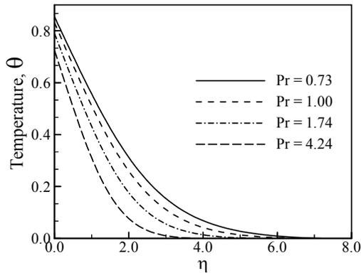
Fig 4: Variation of temperature profiles for different values of  $Pr$  with  $Q = 0.01$
