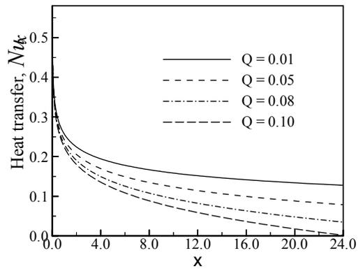
Fig 7: Variation of rate of heat transfer for different values of  $Q$  with  $Pr = 0.73$
