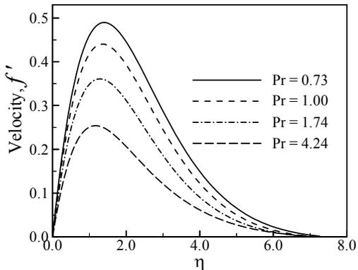
Fig 5: Variation of velocity profiles for different values of  $Pr$  with  $Q = 0.01$
