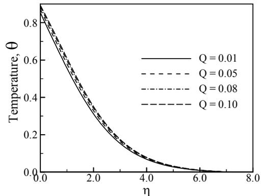
Fig 2: Variation of temperature profiles for different values of  $Q$  with  $Pr = 0.73$
