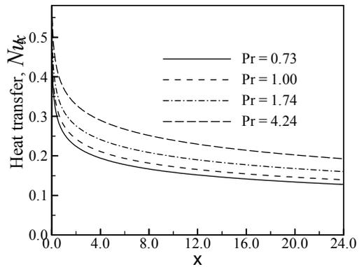
Fig 9: Variation of rate of heat transfer for different values of  $Pr$  with  $Q = 0.01$
