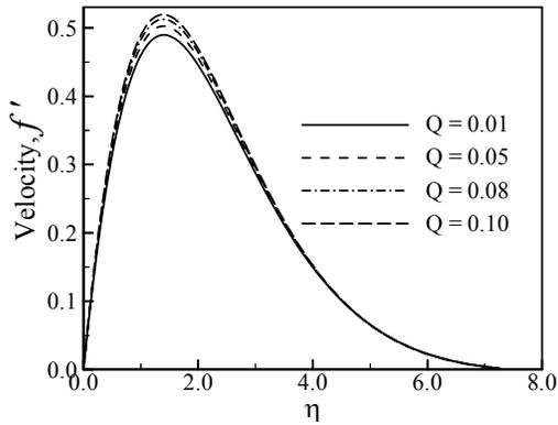
Fig 3: Variation of velocity profiles for different values of  $Q$  with  $Pr = 0.73$
