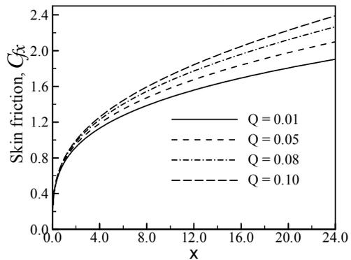
Fig 6: Variation of skin friction coefficients for different values of  $Q$  with  $Pr = 0.73$
