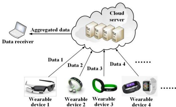
Fig. 6 Architecture of cloud-assisted wireless wearable communications
